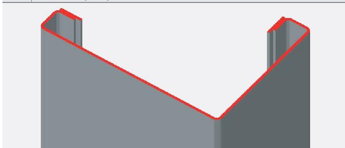
2 Design of the corner profiles allows to erect buildings up to three floors
